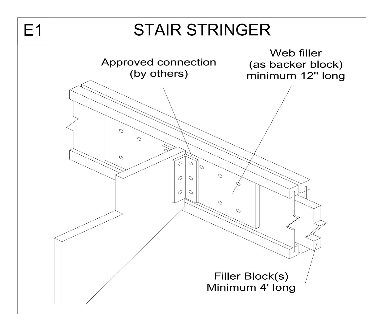
See I-Joist Header Design for connection information of the filler and backer blocks See I-Joist Filler Schedule for filler block and web filler sizes
