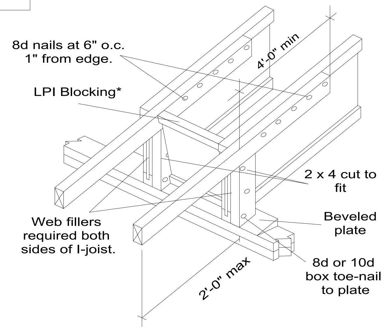
\* Lateral resistance shall be provided. Other methods of restraint, such as full depth LP® SolidStart® OSB Rim, LSL, or LVL may be substituted for the LPI blocking shown.
