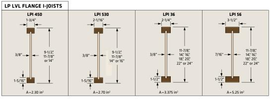
Where A=the cross-sectional area of a flange
