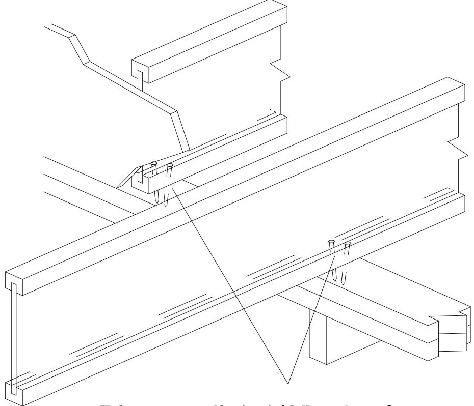
Place nail 1-1/2" min. from end of I-Joist. If nails are close to edge of plate, drive at an angle to reduce splitting.
