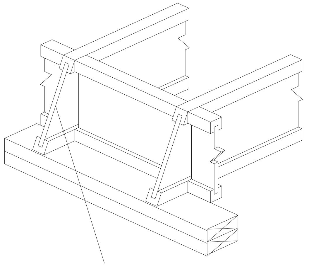
Bevel cut may not extend beyond inside face of bearing wall
