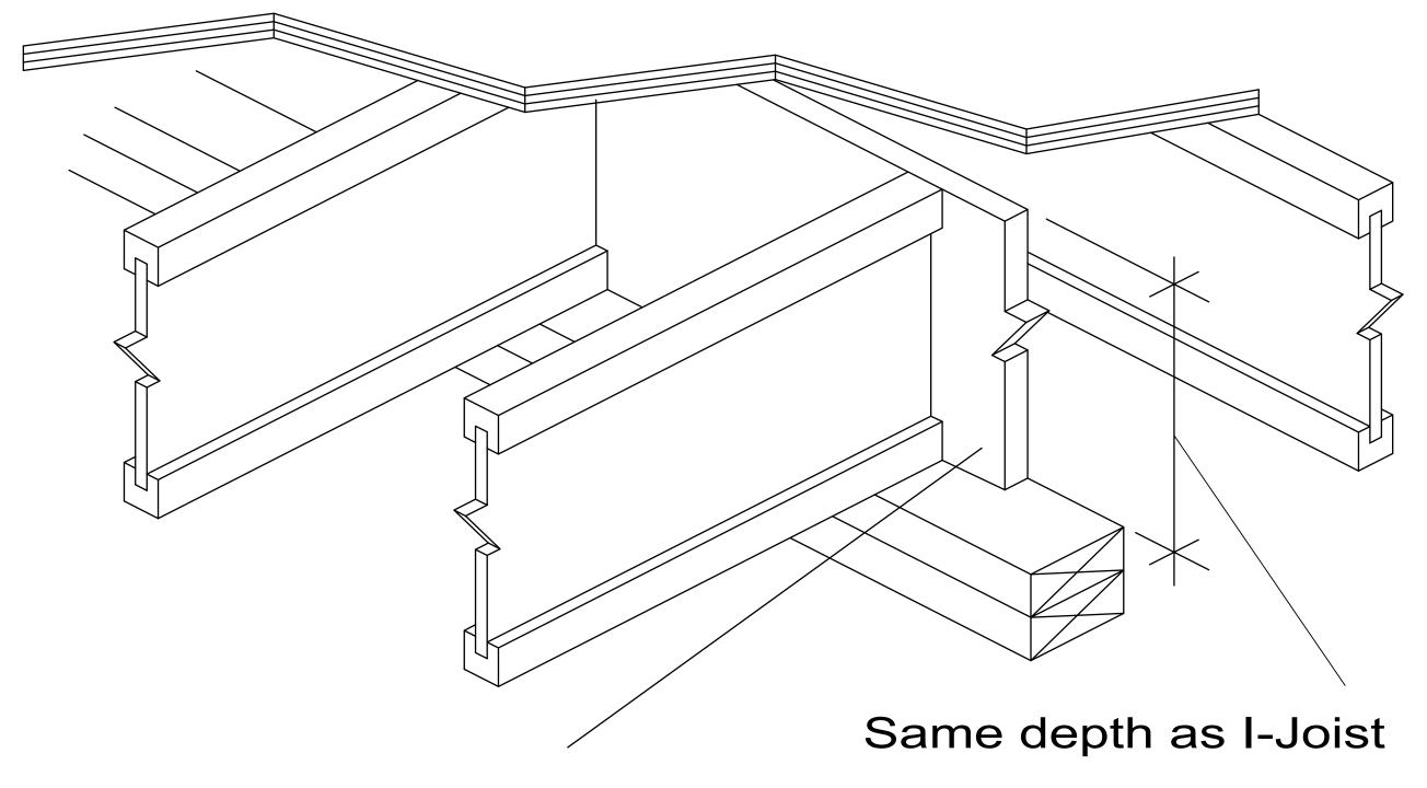
10d box nails at 6" oc toe-nailed from side away from I-Joists
