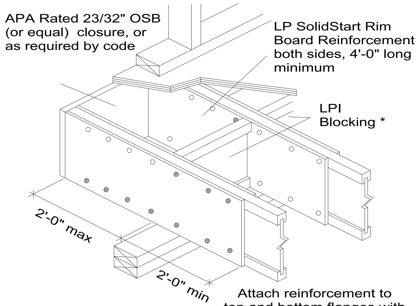
\* LPI SolidStart OSB or LSL Rim Board may be used as Blocking Attach reinforcement to top and bottom flanges with 8d nails at 6" o.c. both sides with nails staggered to avoid splitting
