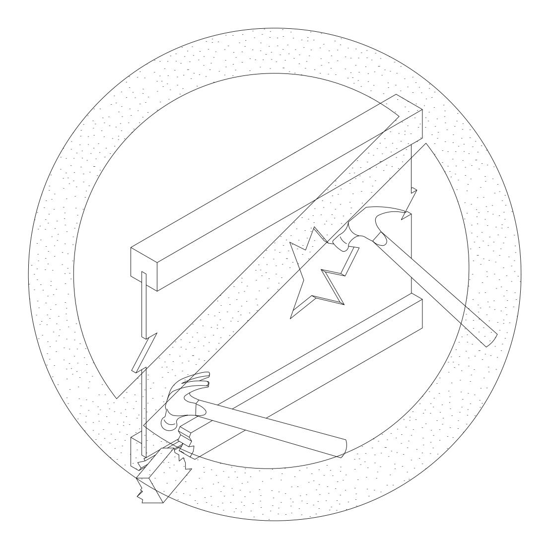
DON'T hammer on flange and damage joist.
