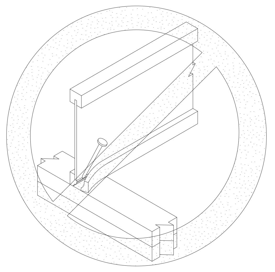
Refer to Joist End Nailing detail, A5, for correct sizes and locations.
