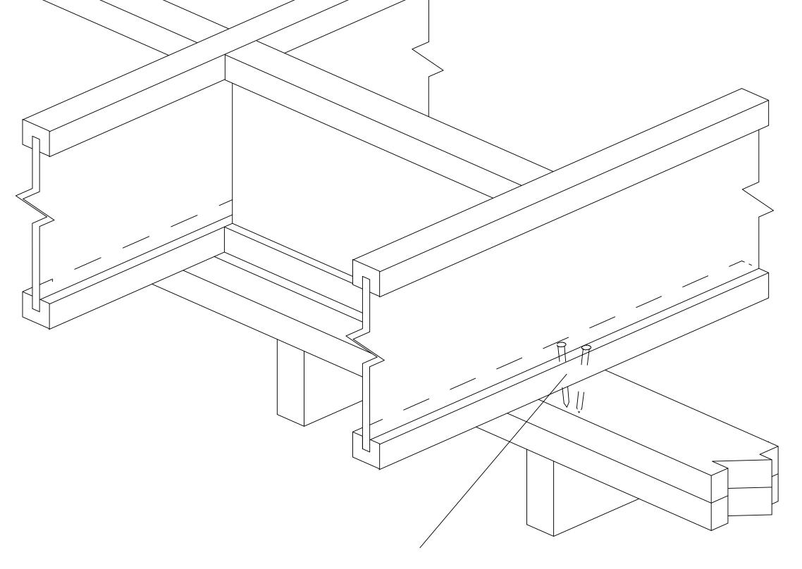
If nails are close to edge of plate, drive at an angle to reduce splitting.
