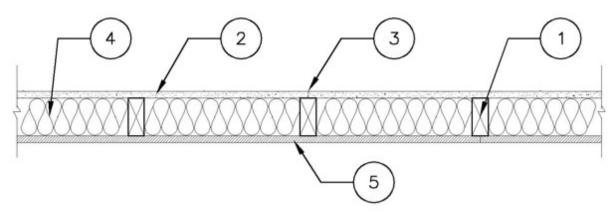
1. **Wood Studs** — Nom 2 by 4 in., spaced 16 in. OC with double 2 by 4 top and single 2 by 4 in, bottom plates. Studs effectively firestopped.
