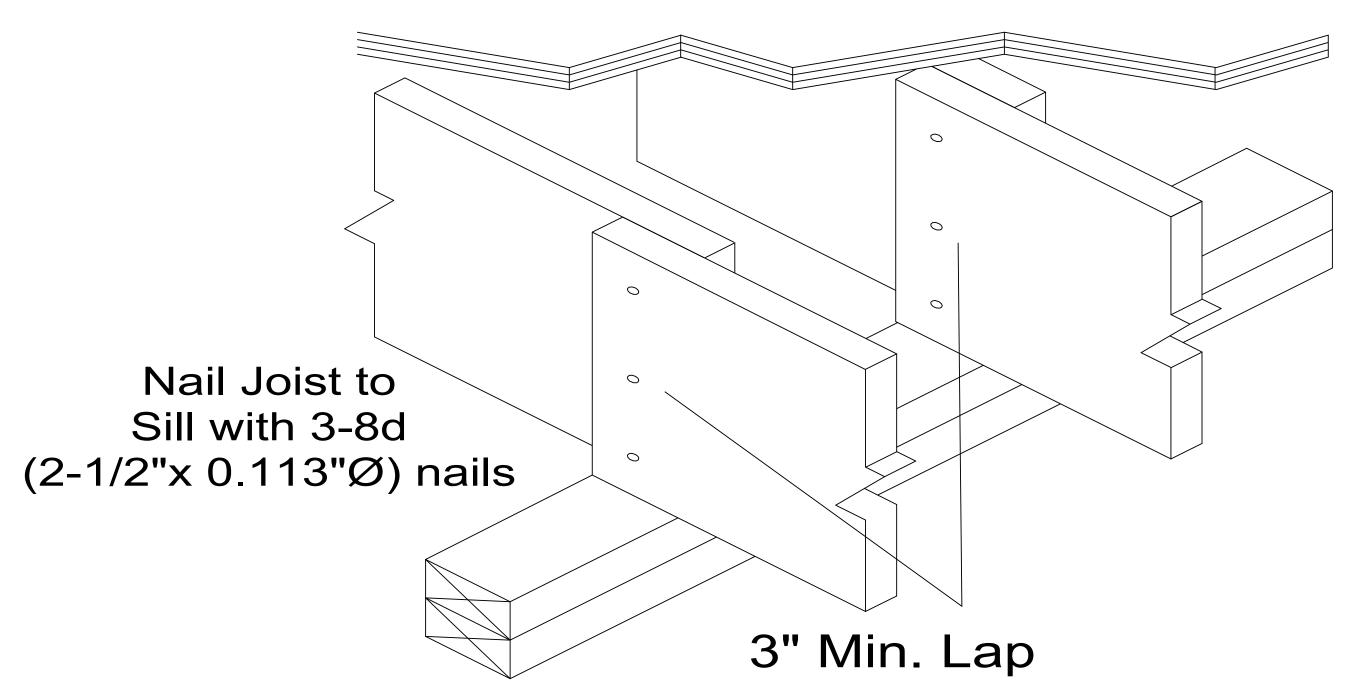
Nail Joists together with a minimum of Three (3) 10d Face Nails
