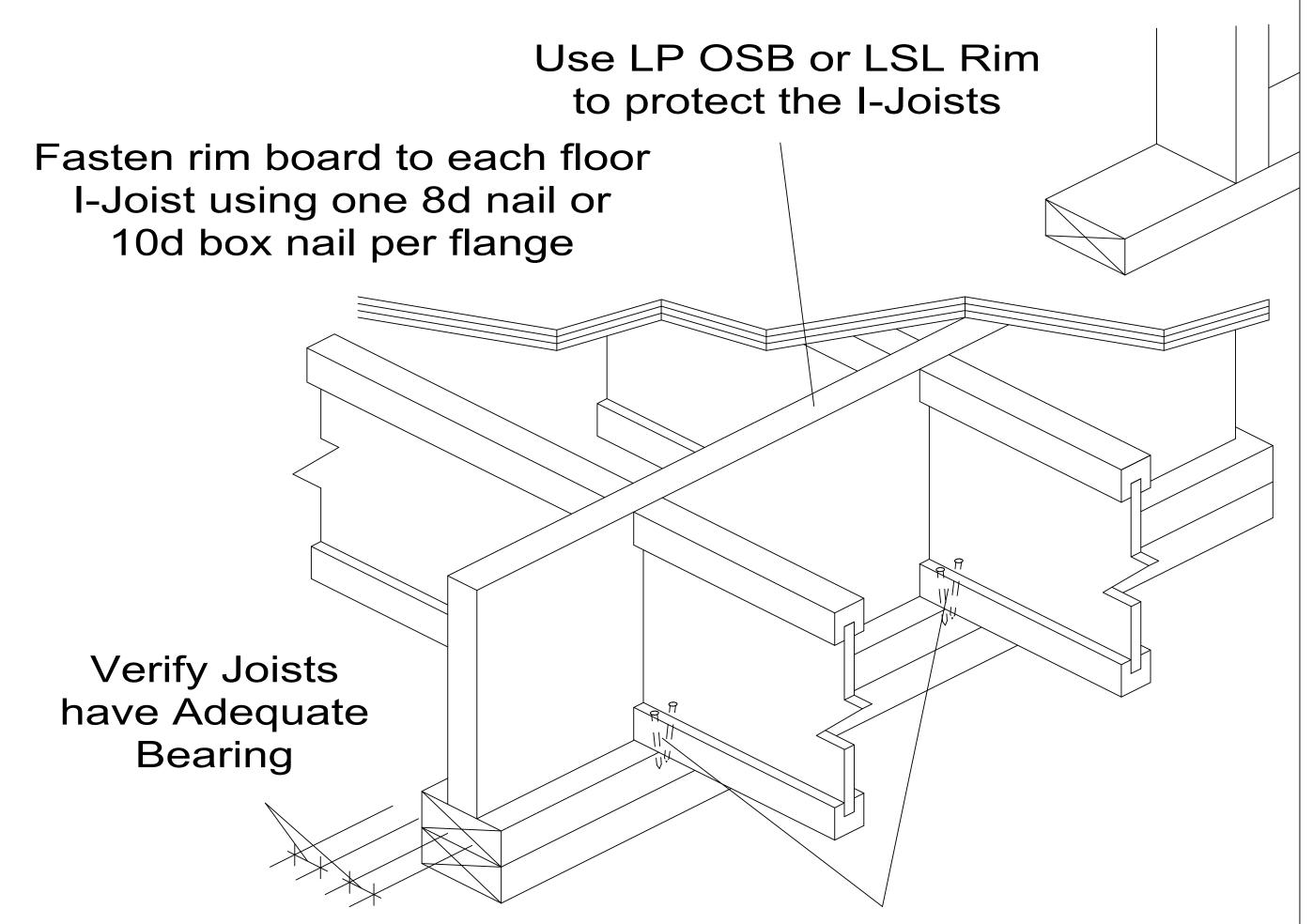
8d nail at 6" o.c. (when used for shear transfer nail to bearing plate with same nailing schedule as decking)
