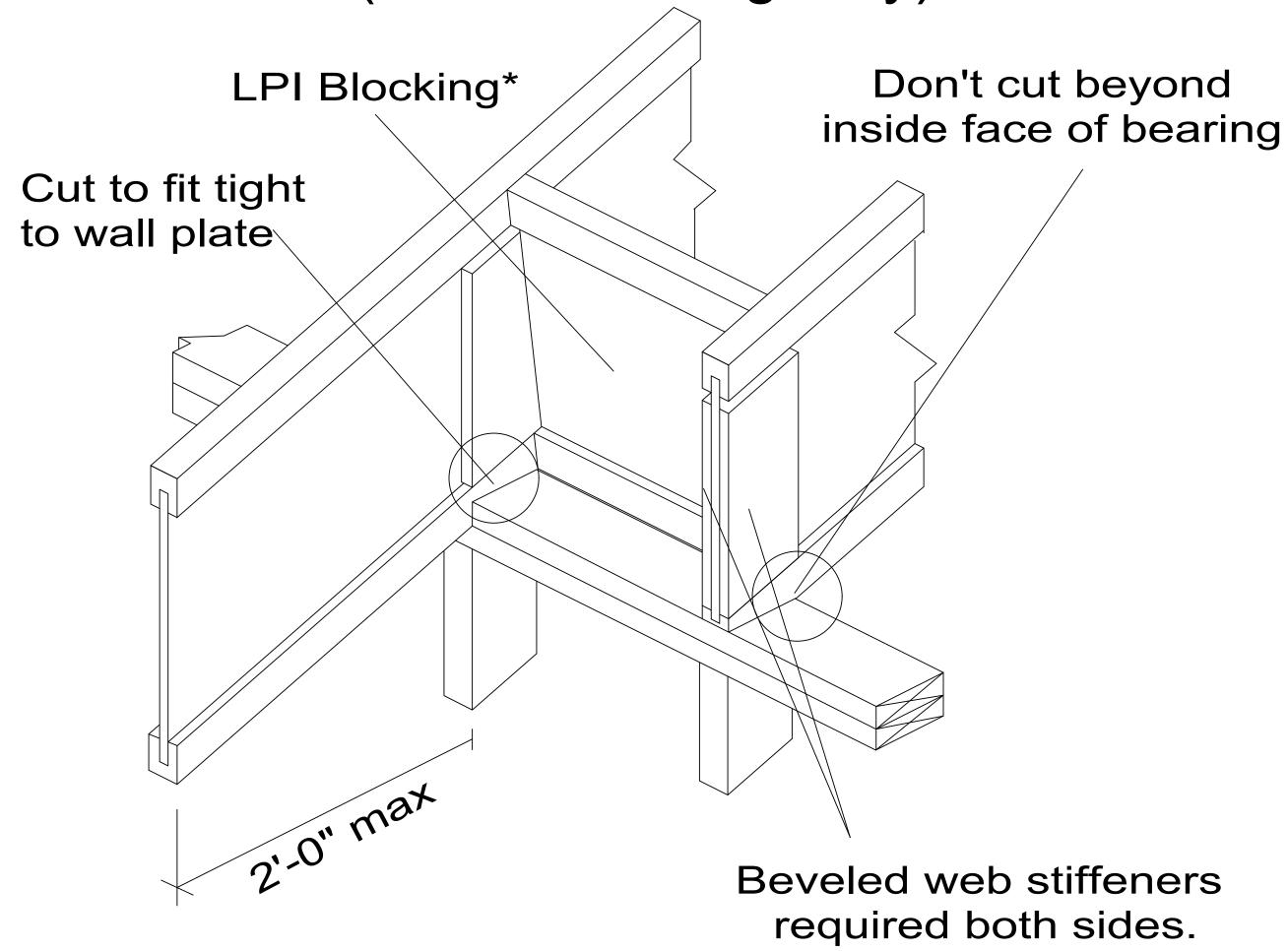
\* Lateral resistance shall be provided. Other methods of restraint, such as full depth LP® SolidStart® OSB Rim, LSL, or LVL may be substituted for the LPI blocking shown.
