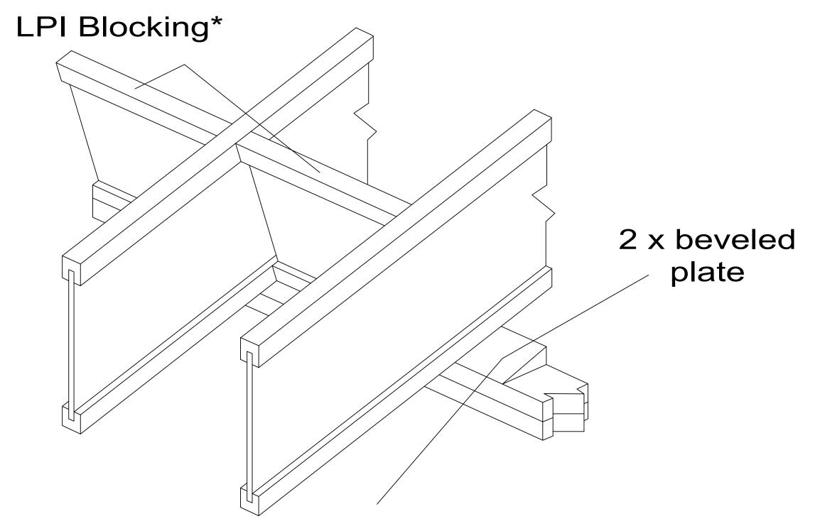
Simpson® VPA, USP® TMP, (or equal) connector may be subsituted for beveled plate. Use of flat bearings or non-sloped hangers with sloped members is acceptable provided that the member pitch is less then or equal to 1/2" rise for 12" of run (0.5:12) or 2.39° degrees. Hanger design is the responsibility of the designer.
