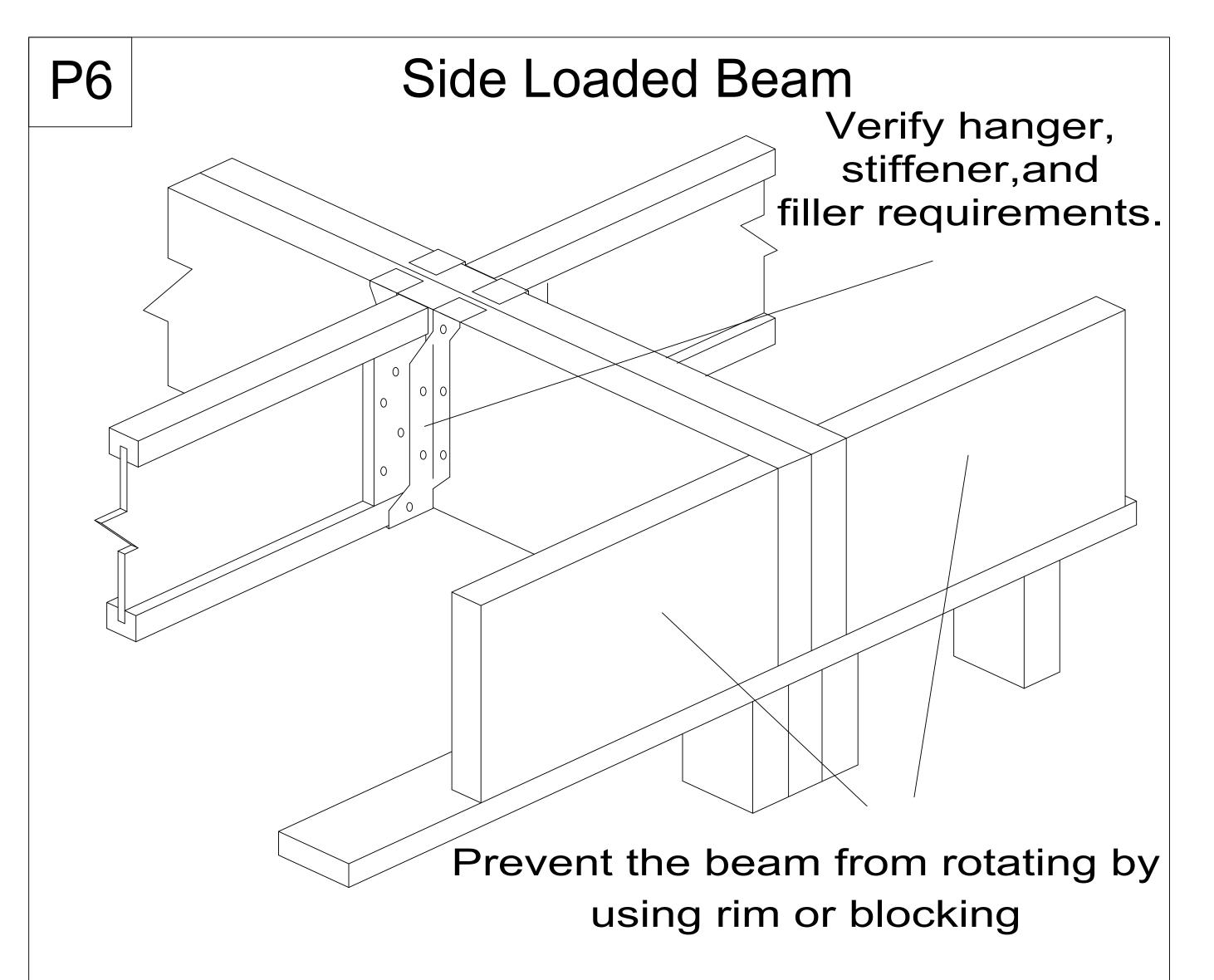
Refer to Connection Assemblies for Multi-Ply connection information. Side loads are not recommended for beams over 5-1/2" wide unless loads are equally applied to both faces.
