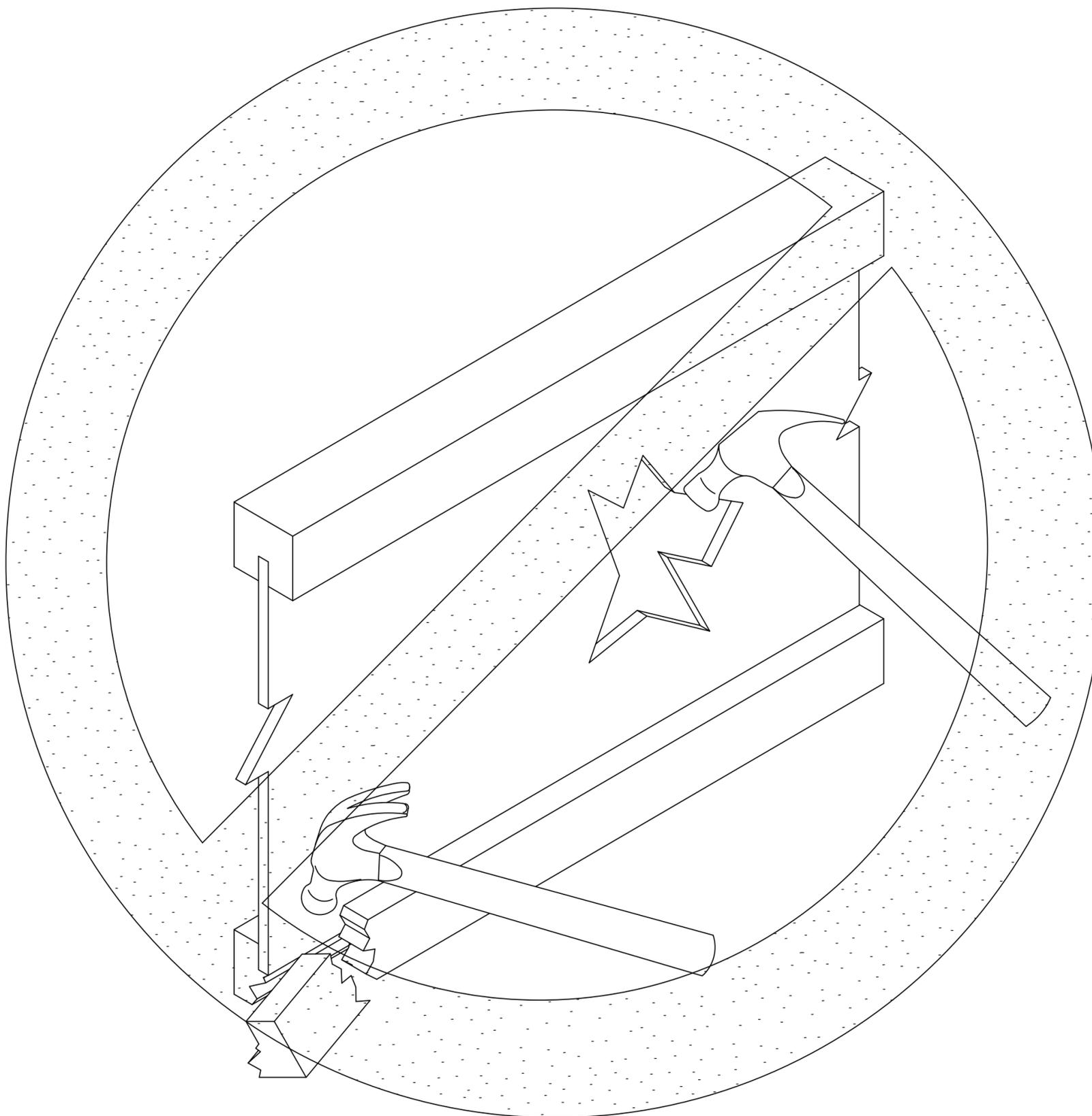
**DON'T** hammer on flange and damage joist.
